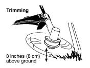
SCALPING - The scalping technique removes unwanted vegetation down to the ground. Hold the bottom of the trimmer head about 3 inches (8 cm) above the ground and at an angle. Allow the tip of the line to strike the ground around trees, posts, monuments, etc. This technique increases line wear.
